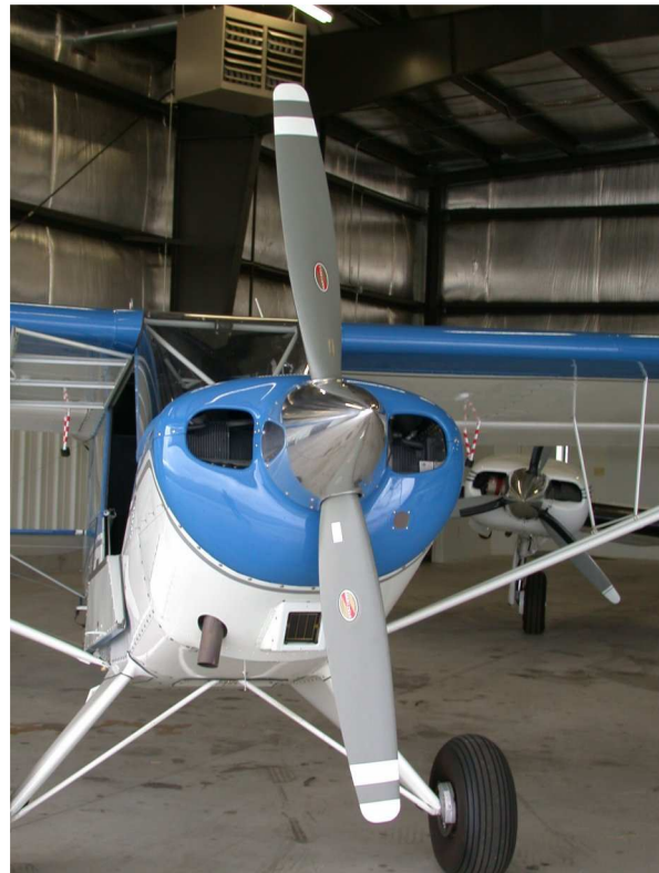
Husky A-1B with Aero Mark's Hartzell 80" Propeller STC.
